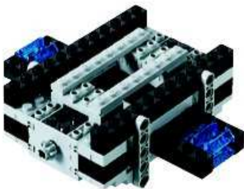
Figure 3: Subassemblies - a vehicle chassis and a pluggable module with two contact sensors.
