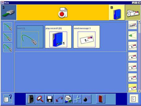
This is the programming of the "robot-friend", in which at a certain degree of bending of the bend sensor, the tape recorder emits a sound to call the "bread-carrier" robot, to which a message in the form of an infrared signal is associated.
