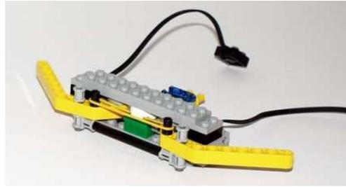
Figure 2. The touch-sensor sub-assembly
