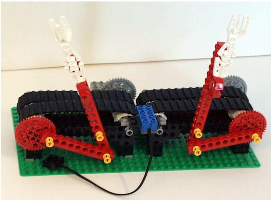
*Figure 17. A modular mechanism for oscillating (waving) motion*
