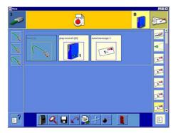
This is the programming of the "robot-friend", in which at a certain degree of bending of the bend sensor, the tape recorder emits a sound to call the "bread-carrier" robot, to which a message in the form of an infrared signal is associated.
