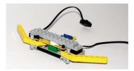
Figure 2. The touch-sensor sub-assembly
